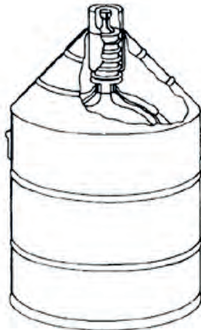
Figure 4: Typical vacuum jacketed Dewar
